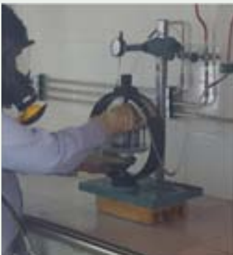
SULPHIDE STRESS CORROSION CRACKING TEST AS PER NACE TM --0177
