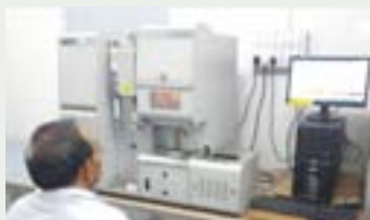
CARBON AND SULPHUR ANALYSIS BY LECO MACHINE
